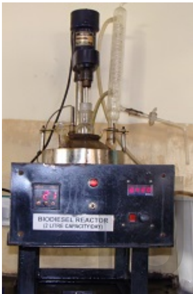
Figure 2. Biodiesel Reactor 1 liter capacity per day
